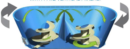
Gray arrows indicate direction of screw rotation. Green arrows indicate Balanced Flow™ of feed
