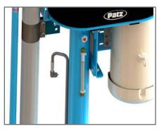
Bearing seals can be purged every 8 hours due to a grease line.
