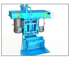
Easy lubrication with convenient oil and grease lines. A **transparent oil line** makes reading oil levels simple.
