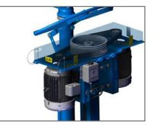
The **belt drive system** creates less stress on the upper drive shaft and bearings.
