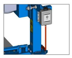
A transparent oil reservoir makes reading oil levels simple. A large fill hole makes adding oil easy.
