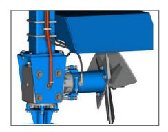
An adjustable shear plate, located close to the propeller, breaks up dried or frozen maure for a more homogenous slurry.
