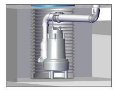
The "sump" is a poly container that the pump sits in. Liquid gets directed here from the gutter.
