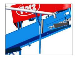
**Pipe supports the PVC along the slide** of the material mover or gutter cleaner. Supports are recommended every 10' (3m).
